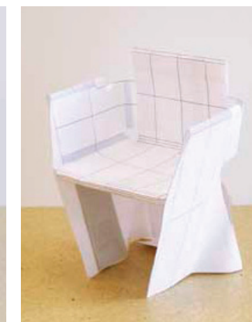
IDEAS WERE REJECTED AND FURTHER DEVELOPED USING A ONE-FIFTH SCALE CARDBOARD MODEL. THE HEIGHT AND FORM OF THE BACKREST ARE DEFINED.
